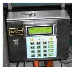
back to the spectrometer where the component concentrations are calculated. The data is displayed on the Remote Display Module, which can be mounted at a convenient position for use by an operator. Alternatively the system can be operated from our software running on a PC and the data shown in real time in the form of trend charts. 4-20mAmp output signals are also available for supply to other process control equipment. Australian designed and manufactured.
